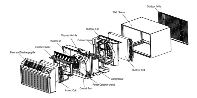
Wall sleeve: all our sleeves have industry standard dimensions of 26" wide x  $15\frac{3}{4}$ " high. The  $16\frac{3}{4}$ " depth is the industry
