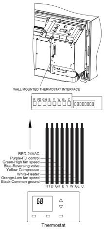
Fig 9 Wall mounted thermostat wiring
