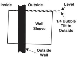
Fig 6 Proper Sleeve Tilt
