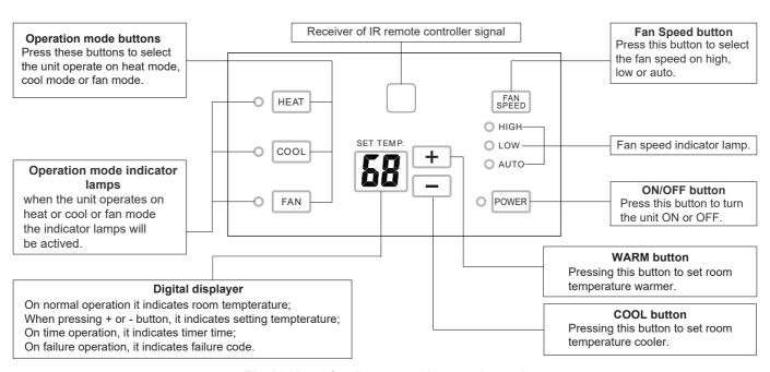
Fig 10 Use of unit mounted control panel
