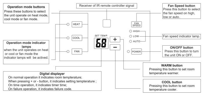
Fig.6-1 Use of unit mounted control panel
