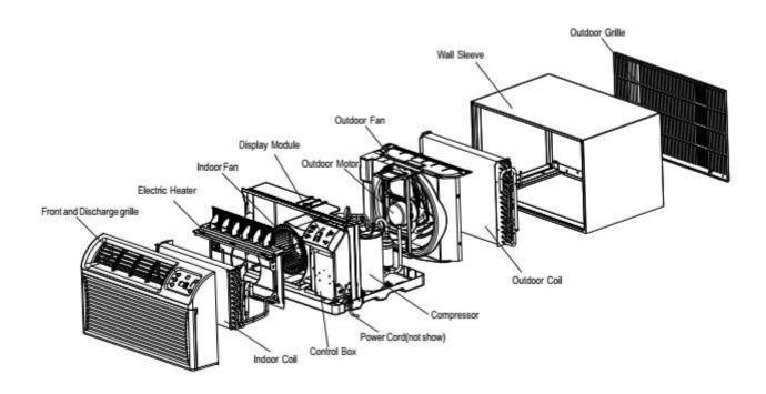
Wall sleeve: all our sleeves have industry standard dimensions of 26" wide x  $15\frac{3}{4}$ " high. The  $16\frac{3}{4}$ " depth is the industry
