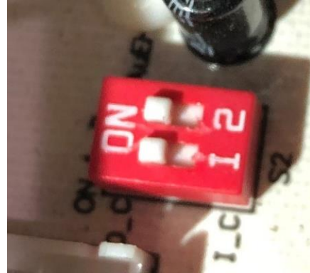
Dip Switch ON (Switch #1)
