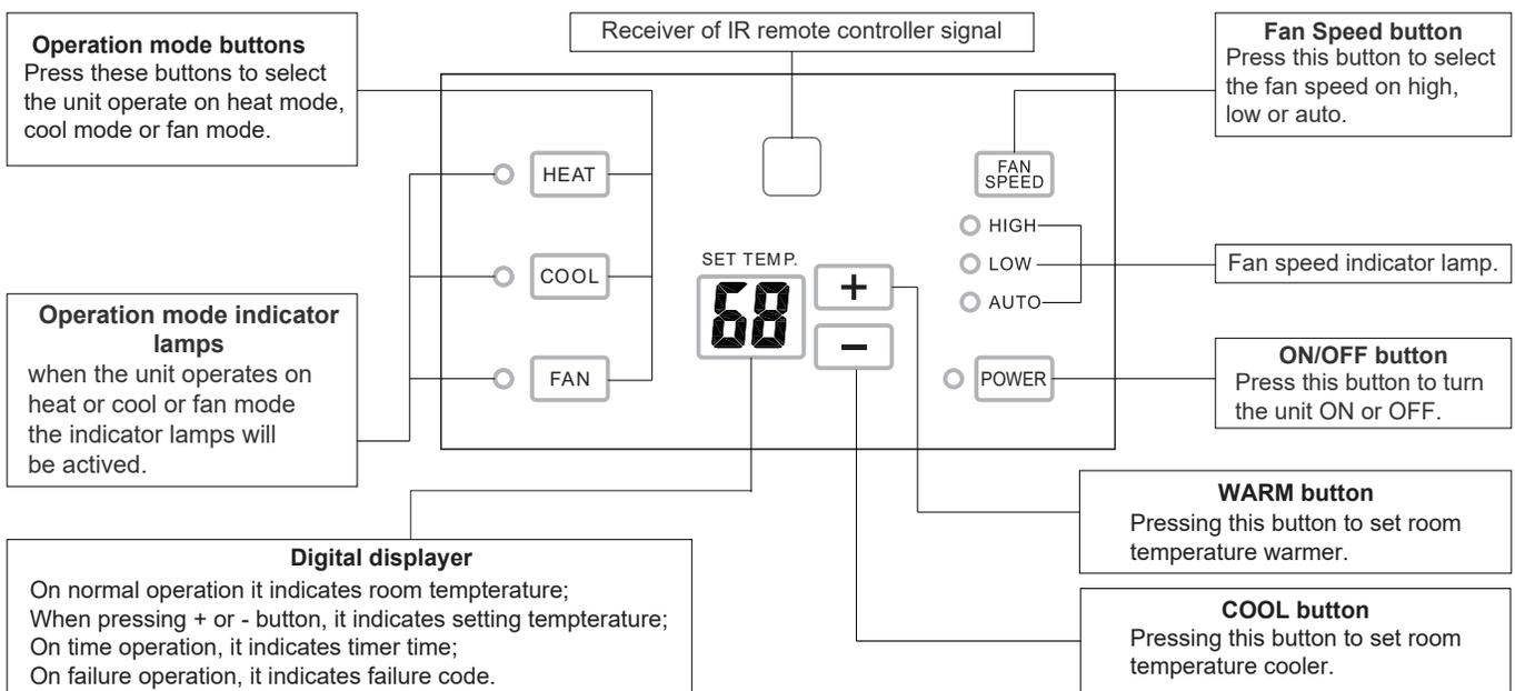
**Fig 10 Use of unit mounted control panel**
