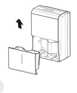
Hold both sides of the bucket with even strength, and pull it out from the unit.
